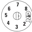
PC mount, no bushing, position numbers molded standard. Shown with '15' actuator; not available with '08' actuator or FCXX models.
